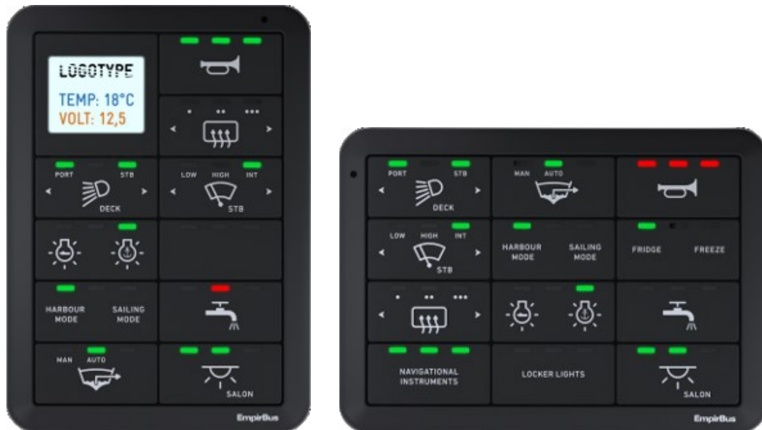
Figure 6.1: SP-12 panels with designed buttons and display
